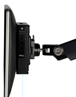
The Verint HDR-P Micro installed on a video monitor with the VESA mount option
